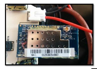
V2.0 used ESP8266, also with no secure storage
